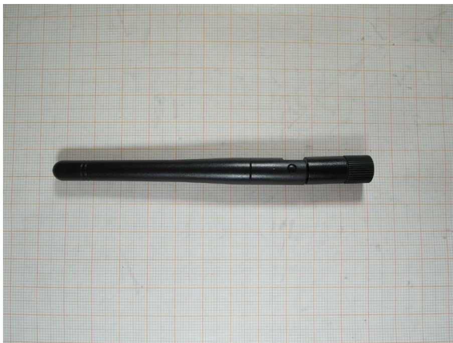
Photo 7: DelockRP-SMA_88395 - antenna 1 - omnidirectional dipole antenna
