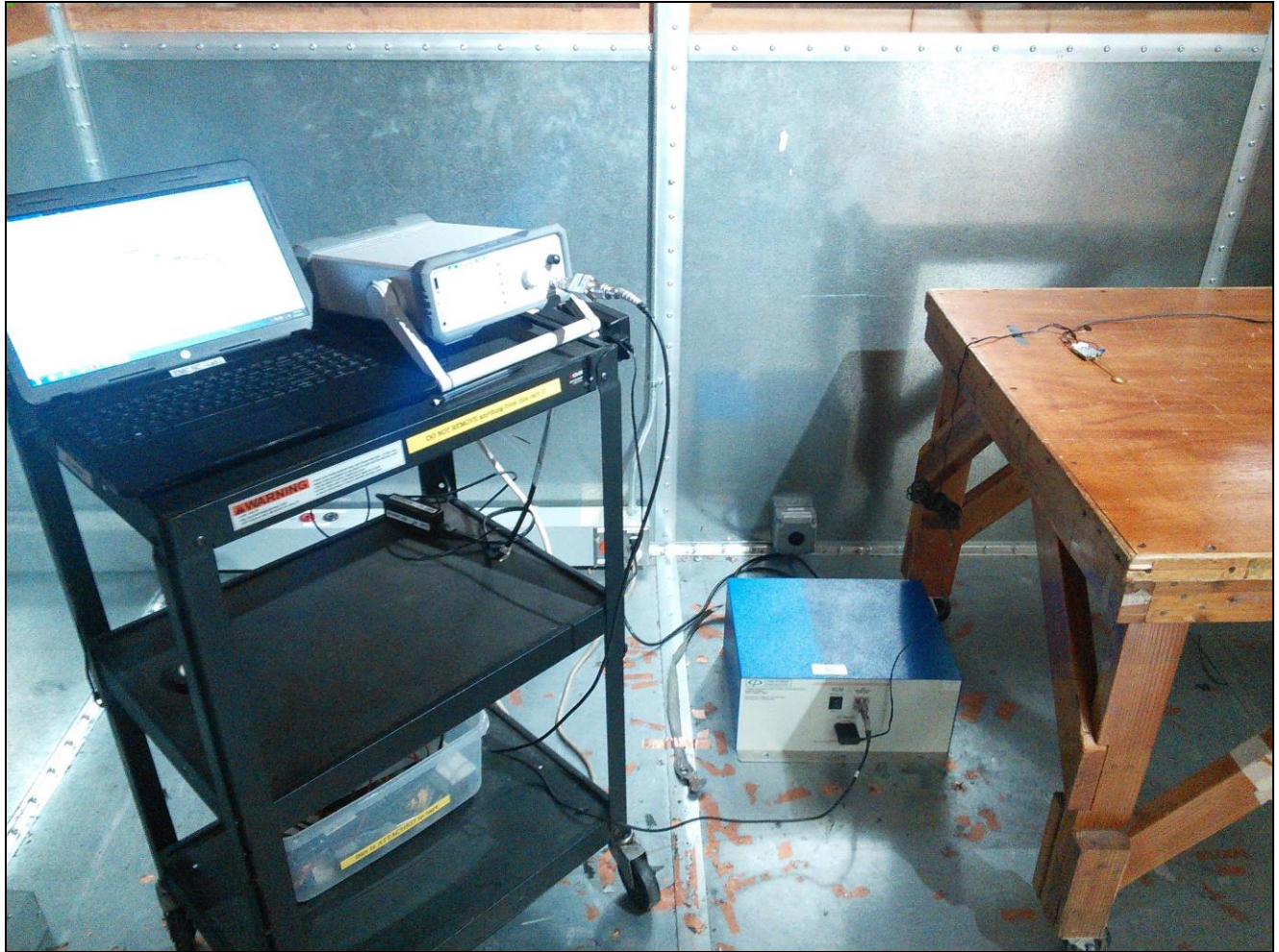
Photograph 1. Conducted Emissions, 15.207(a), Test Setup
