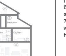
1. Prioritize the installation of a smoke alarm in the bedroom and walkways, and make sure you can hear the alarm from all sleeping areas. In a home with several bedrooms, install an alarm in every bedroom. If you install only one smoke alarm in your home, install the alarm near to all bedrooms where possible, and not in a basement or furnace room.
