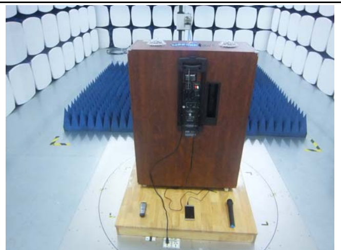
Radiated Emissions Test Setup Above 1GHz
