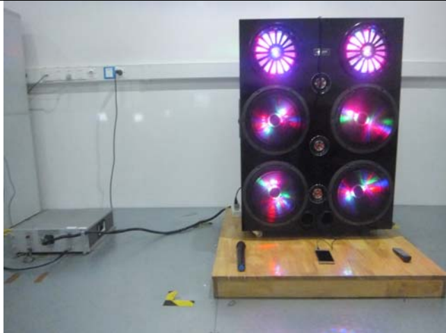
Conducted Emissions Test Setup Front View
