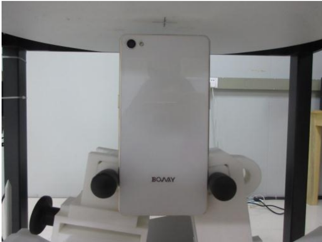
10mm body-worn Top Side Setup Photo(hotspot)
