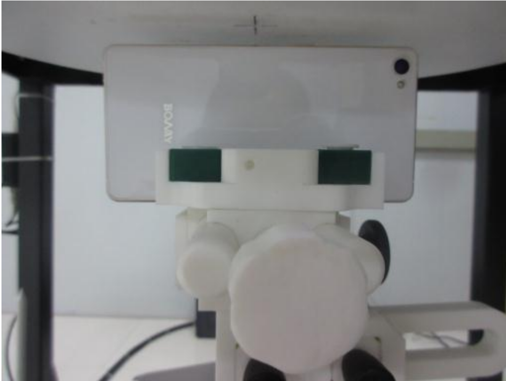
10mm body-worn Right Side Setup Photo(hotspot)
