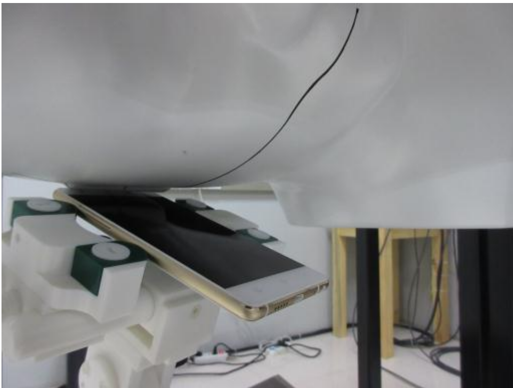
Head Setup Photo(Right Tilt )
