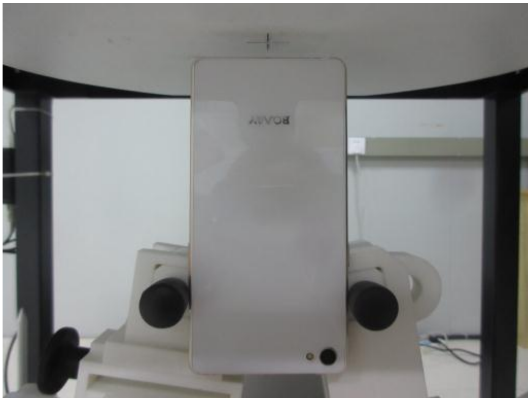
10mm body-worn Bottom Side Setup Photo(hotspot)
