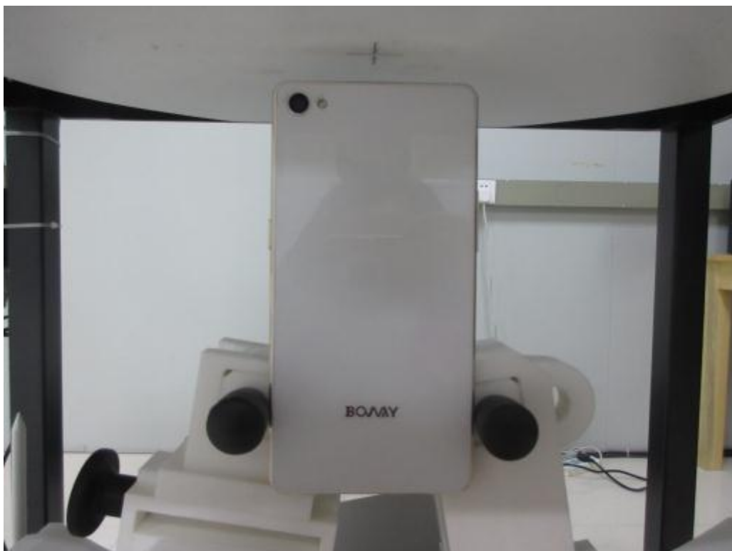
10mm body-worn Top Side Setup Photo (hotspot)
