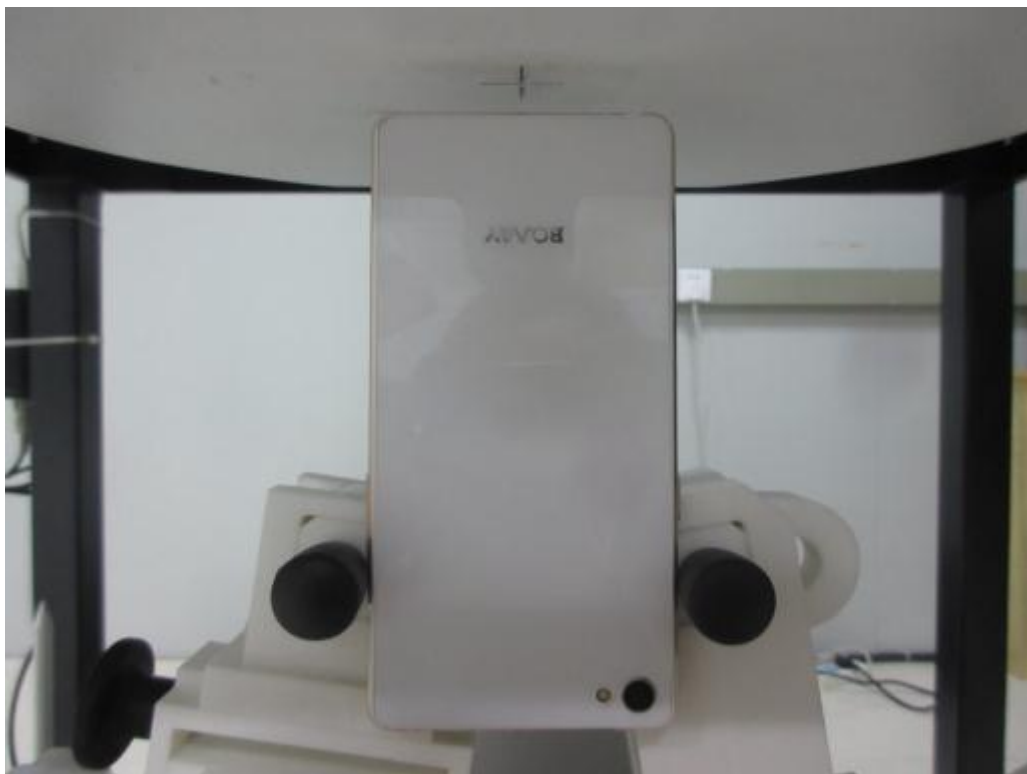
10mm body-worn Bottom Side Setup Photo (hotspot)
