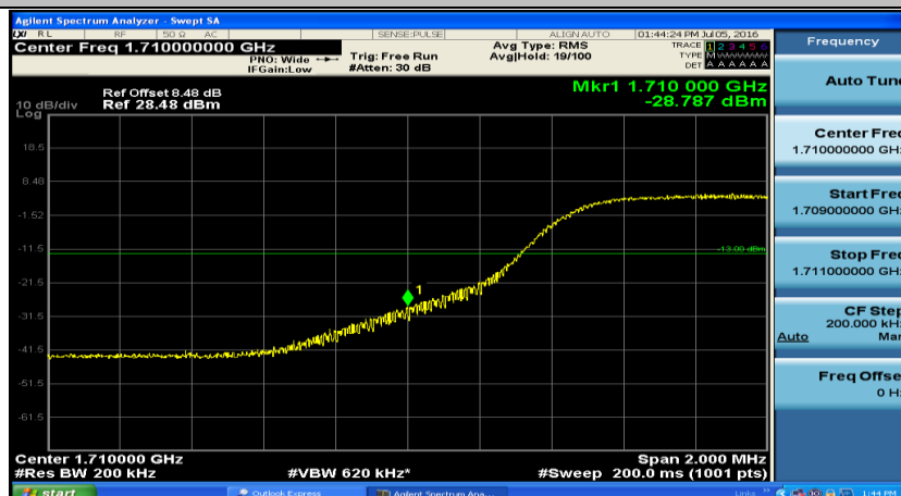
Channel Bandwidth: 10 MHz_HCH_QPSK_1RB#0
