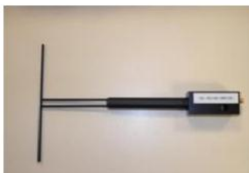
Figure 1 – Satimo COMOSAR Validation Dipole
