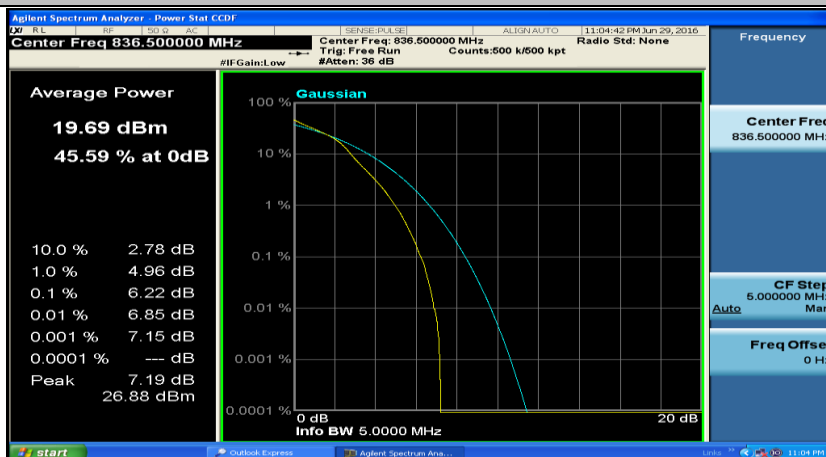
(Channel Bandwidth: 5 MHz)_MCH_16QAM_25RB#0
