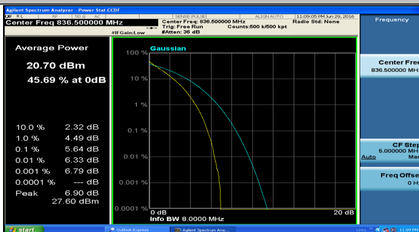
Channel Bandwidth: 10 MHz_MCH_QPSK_50RB#0
