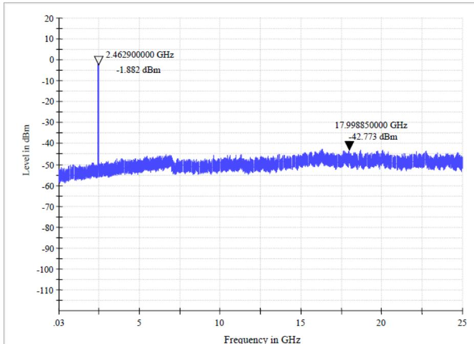
In any 100kHz bandwidth, the Conducted Spurious Emissions from 30 MHz to 25 GHz were greater than 20dB below the peak emission within the band that contains the highest level of the desired power.
