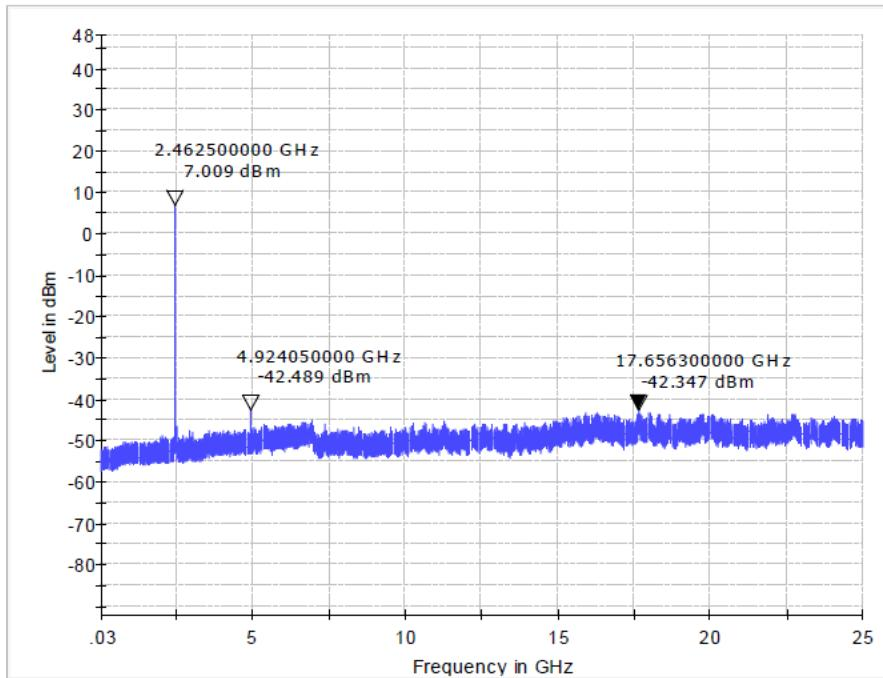
In any 100kHz bandwidth, the Conducted Spurious Emissions from 30 MHz to 25 GHz were greater than 20dB below the peak emission within the band that contains the highest level of the desired power.
