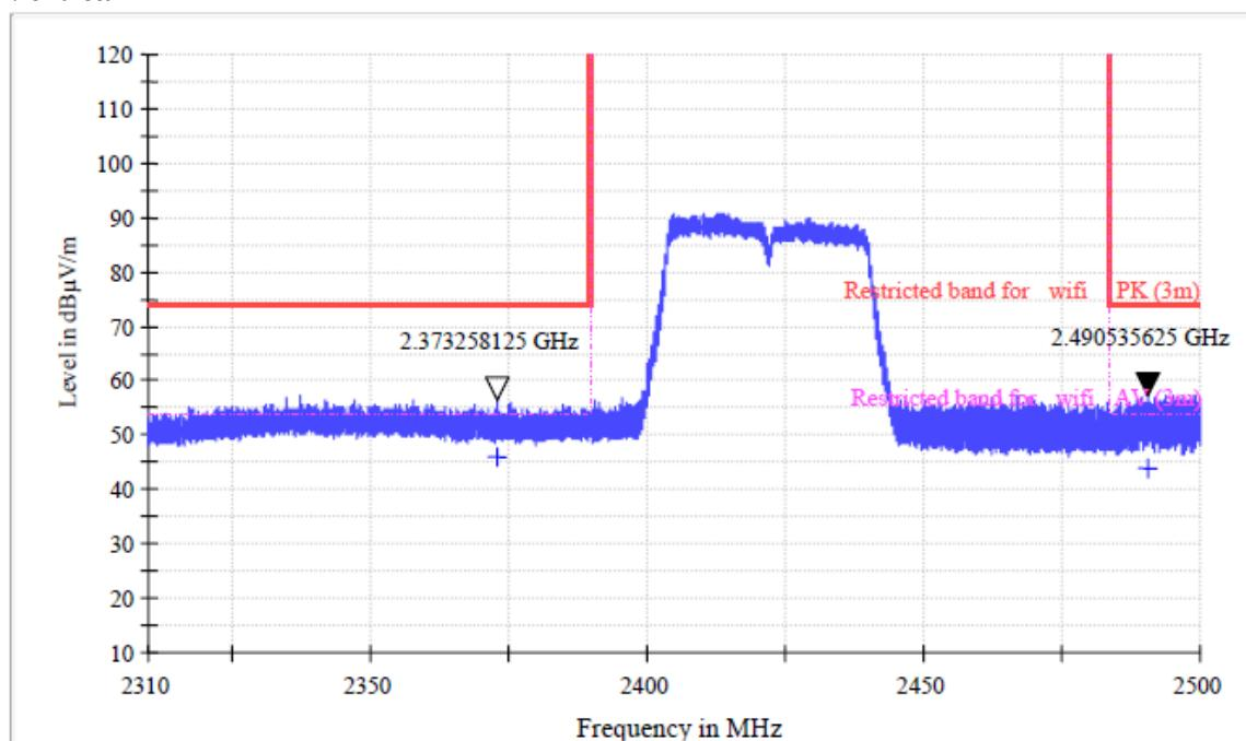
Test at Channel 6 (2.437 GHz) in transmitting status
