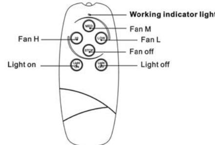
1. Speed control buttons of fan: H.M.and L are speed button.
