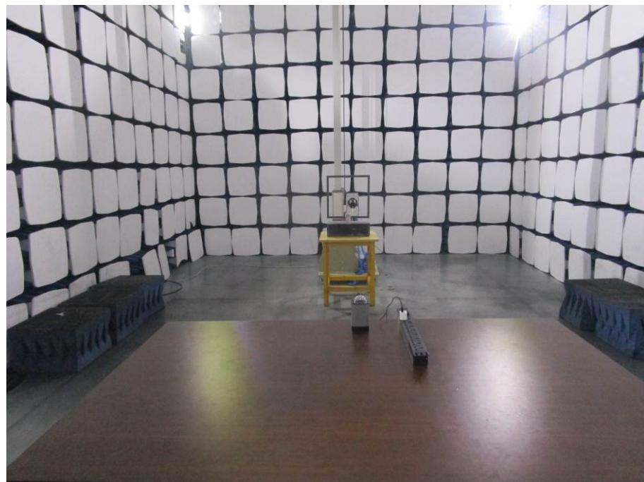
**Radiation Emission Test Setup (30MHz to 1GHz)**
