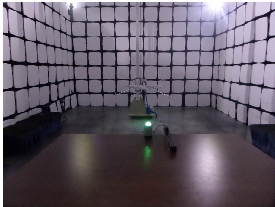
**Radiation Emission Test Setup (Above 1GHz)**
