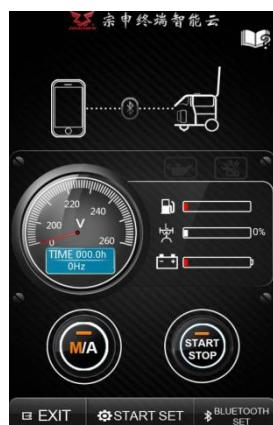
2.3 Connect the power supply of APP controller and keep signal indicator shining. Click BLUETOOTH SET on the right corner of this page to enter blue tooth setup page like this:
