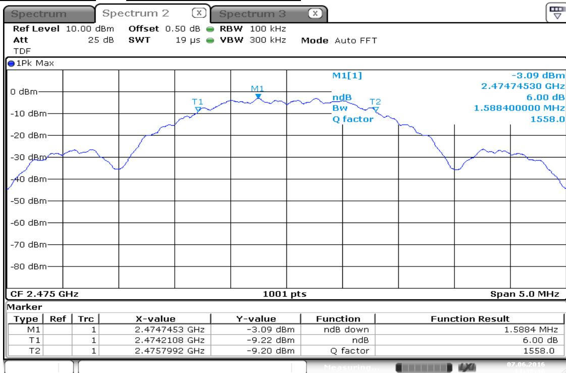
Test mode : RF4CE Ant1\_2 475 MHz\_Occupied Bandwidth
