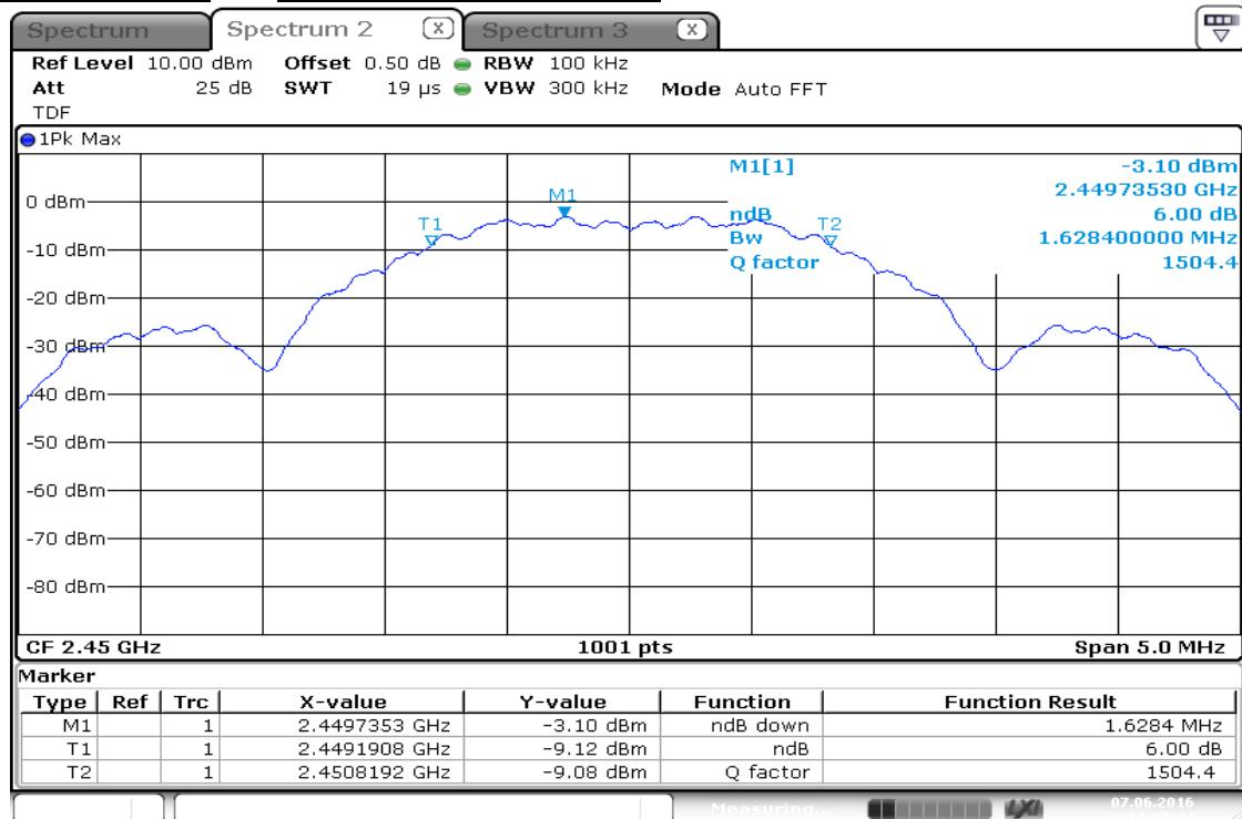
Test mode : RF4CE Ant1\_2 450 MHz\_Occupied Bandwidth
