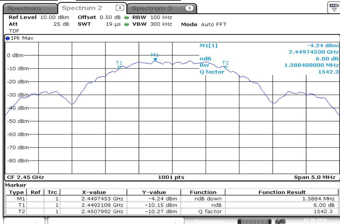
Test mode : RF4CE Ant2\_2 450 MHz\_Occupied Bandwidth
