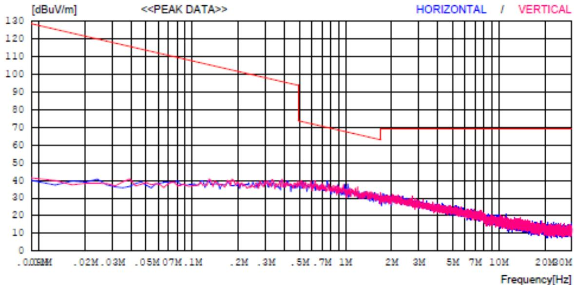
Test mode : 30 MHz ~ 1 GHz ( Worst case : RF4CE Ant1 Lowest Frequency )
