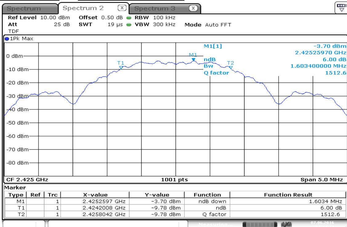
Test mode : RF4CE Ant2\_2 425 MHz\_Occupied Bandwidth
