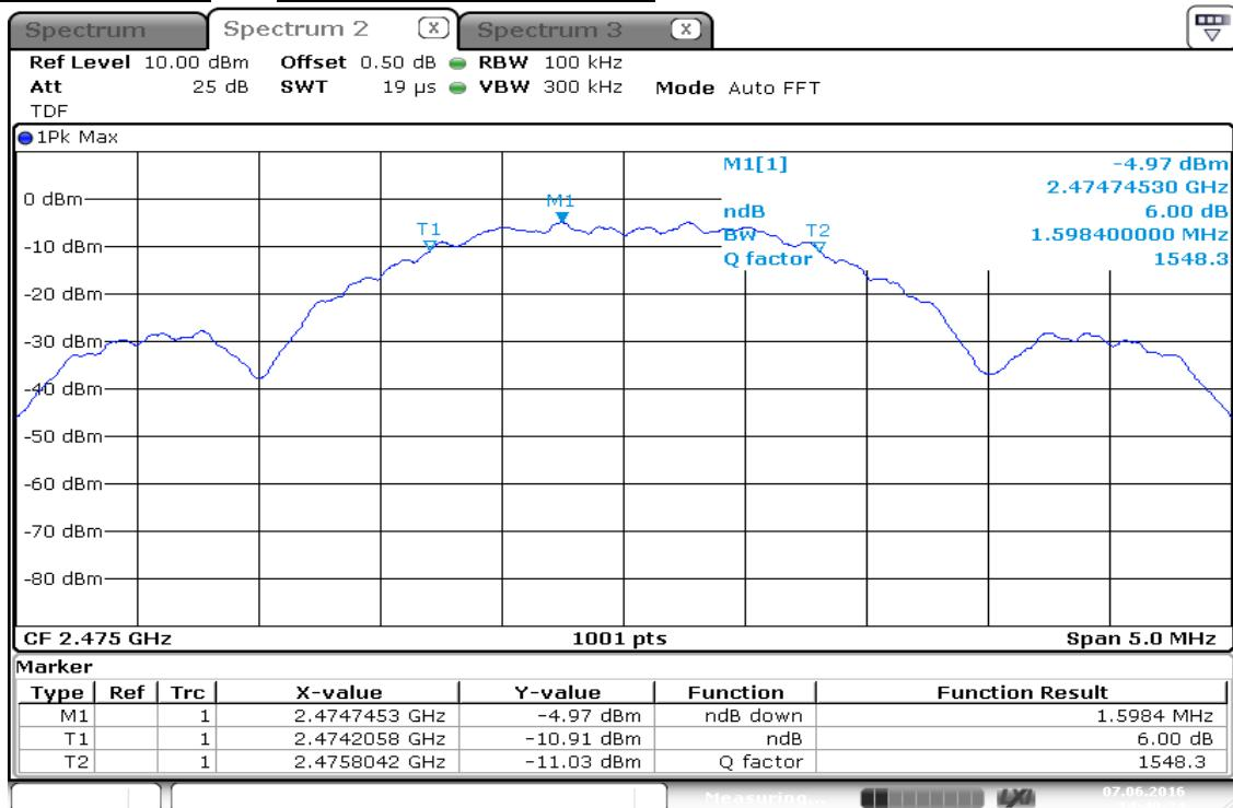
Test mode : RF4CE Ant2\_2 475 MHz\_Occupied Bandwidth
