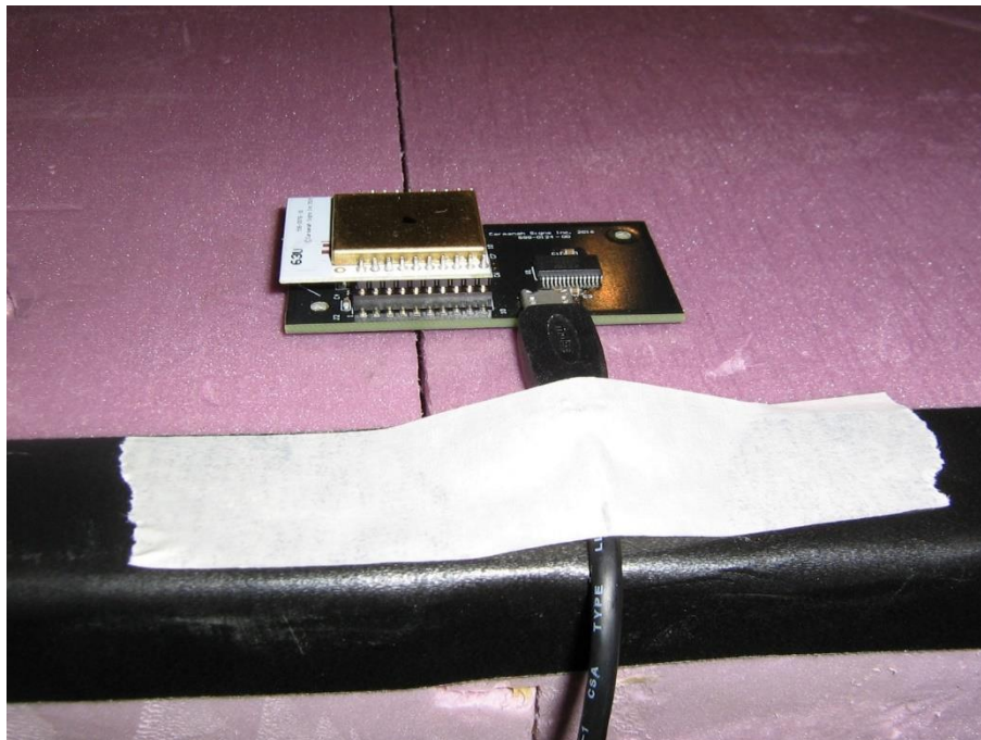
Figure 4: Radiated Spurious Emissions Test Setup (Transmit Mode) at SAC – Vertical on the table top
