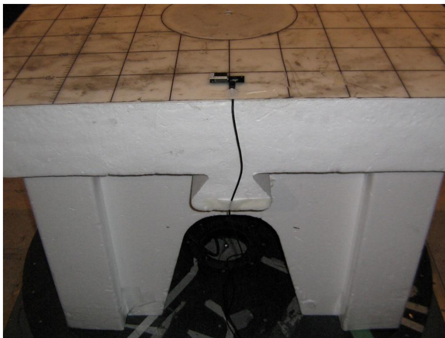
Figure 2: Radiated Spurious Emissions Test Setup (Transmit Mode) at SAC – Flat on the table top
