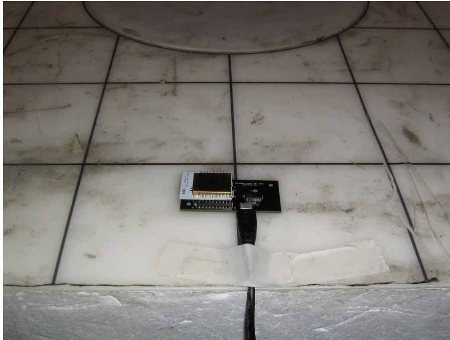
Figure 3: Radiated Spurious Emissions Test Setup (Transmit Mode) at SAC – Flat on the table top
