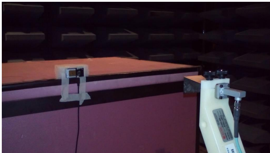
Figure 9: Radiated Spurious Emissions Test Setup (Transmit Mode) from 18-25 GHz at SAC
