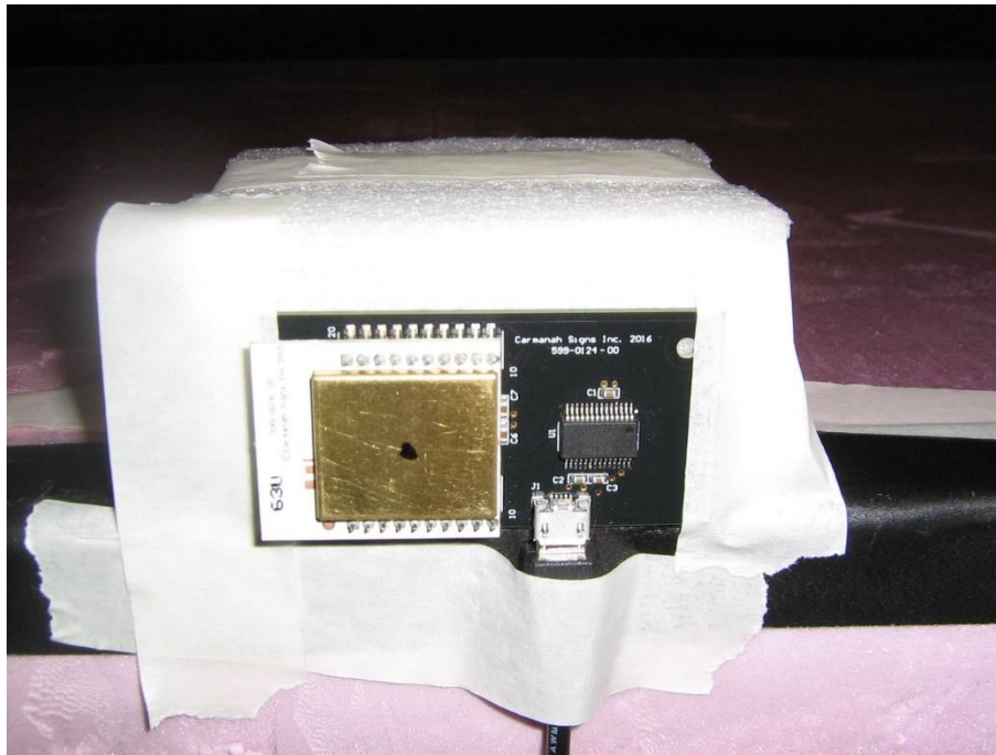
Figure 5: Radiated Spurious Emissions Test Setup (Transmit Mode) at SAC – Vertical and sideways on the table top
