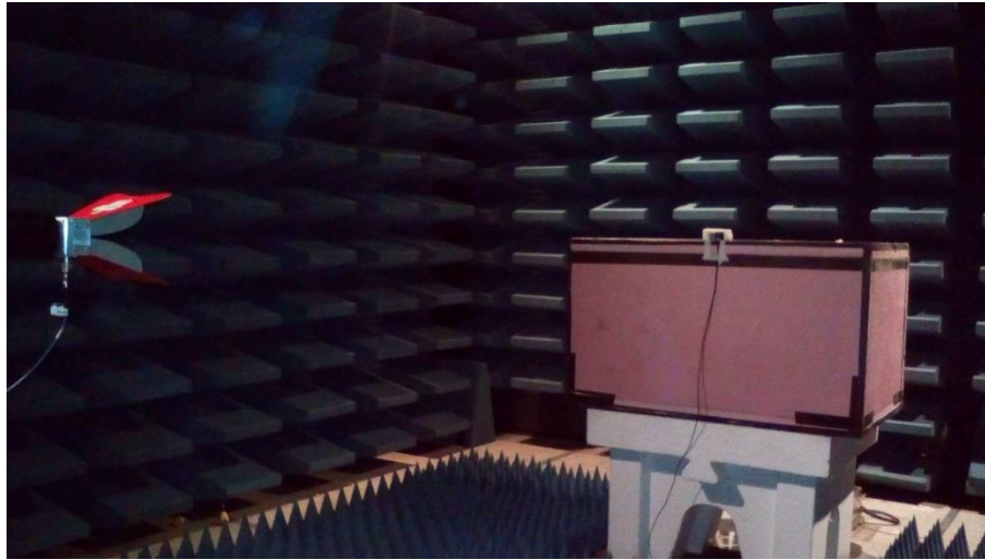
Figure 7: Radiated Spurious Emissions Test Setup (Transmit Mode) from 1-18 GHz at SAC
