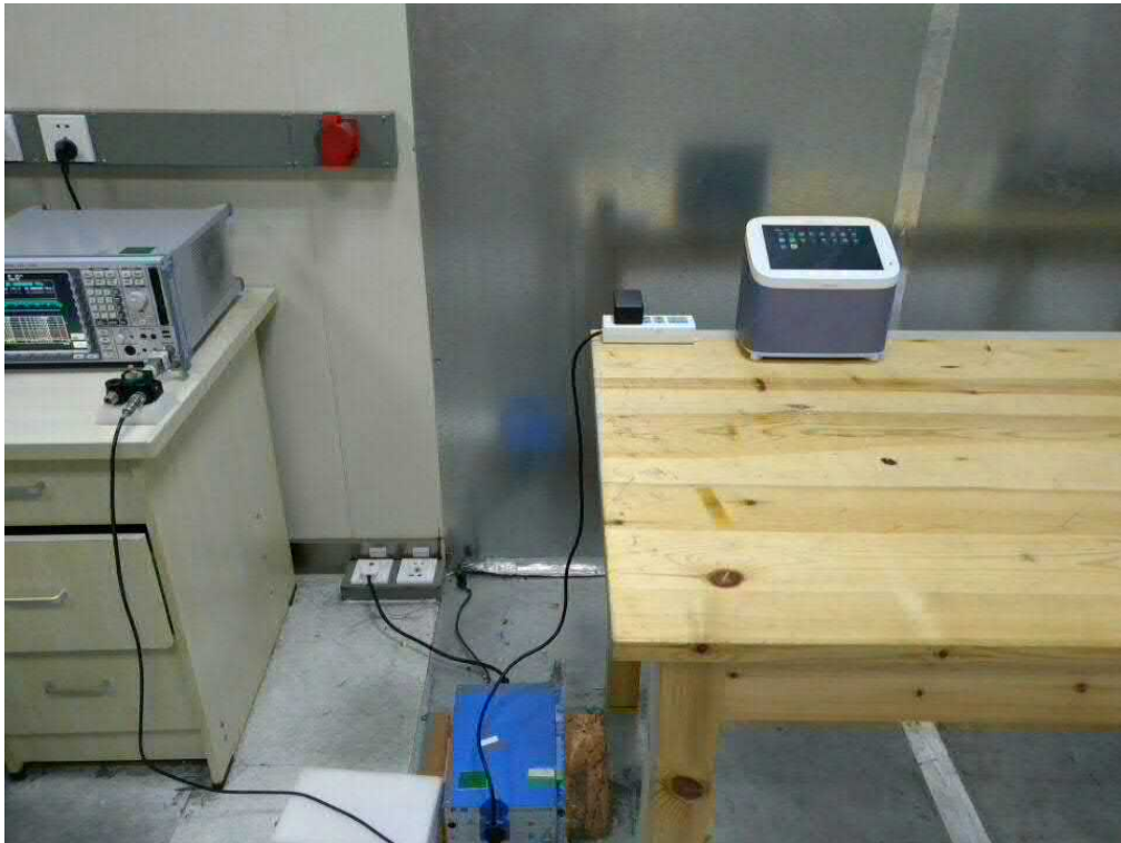
FCC RADIATED EMISSION TEST SETUP BELOW 1GHZ
