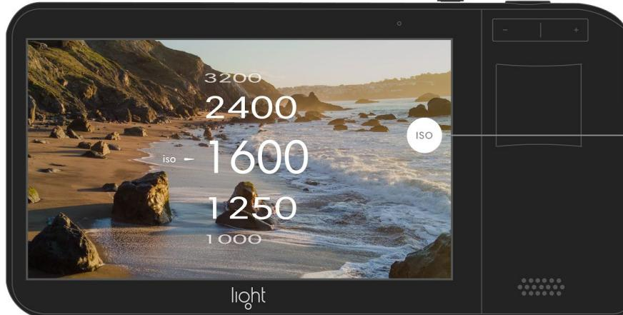
ISO: Press and hold to open ISO slider. Drag up or down to adjust exposure.
