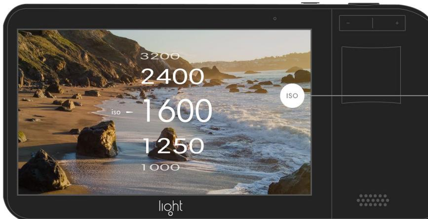
ISO: Press and hold to open ISO slider. Drag up or down to adjust exposure.
