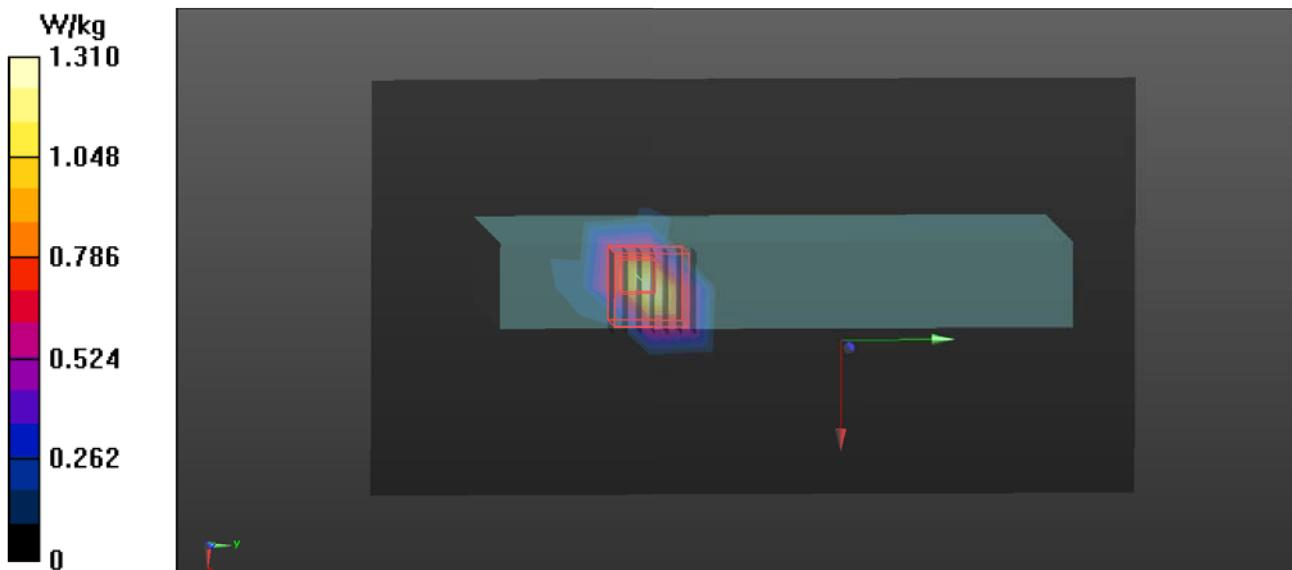
**T73 802.11ac\_VHT40\_Ch149\_Bottom Side\_0.5cm\_Ant 0+1****DUT: FIH;**
