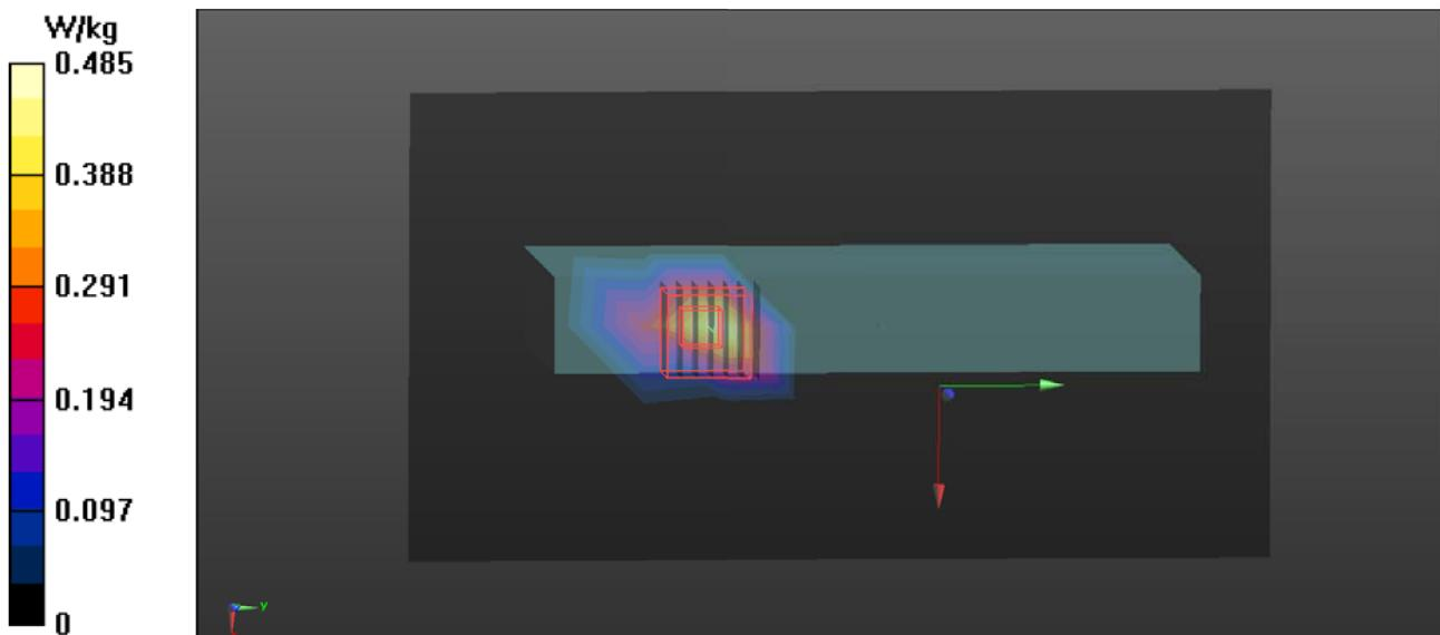
**T20 802.11a\_Ch132\_Bottom Side\_0.5cm\_Ant 0****DUT: FIH;**
