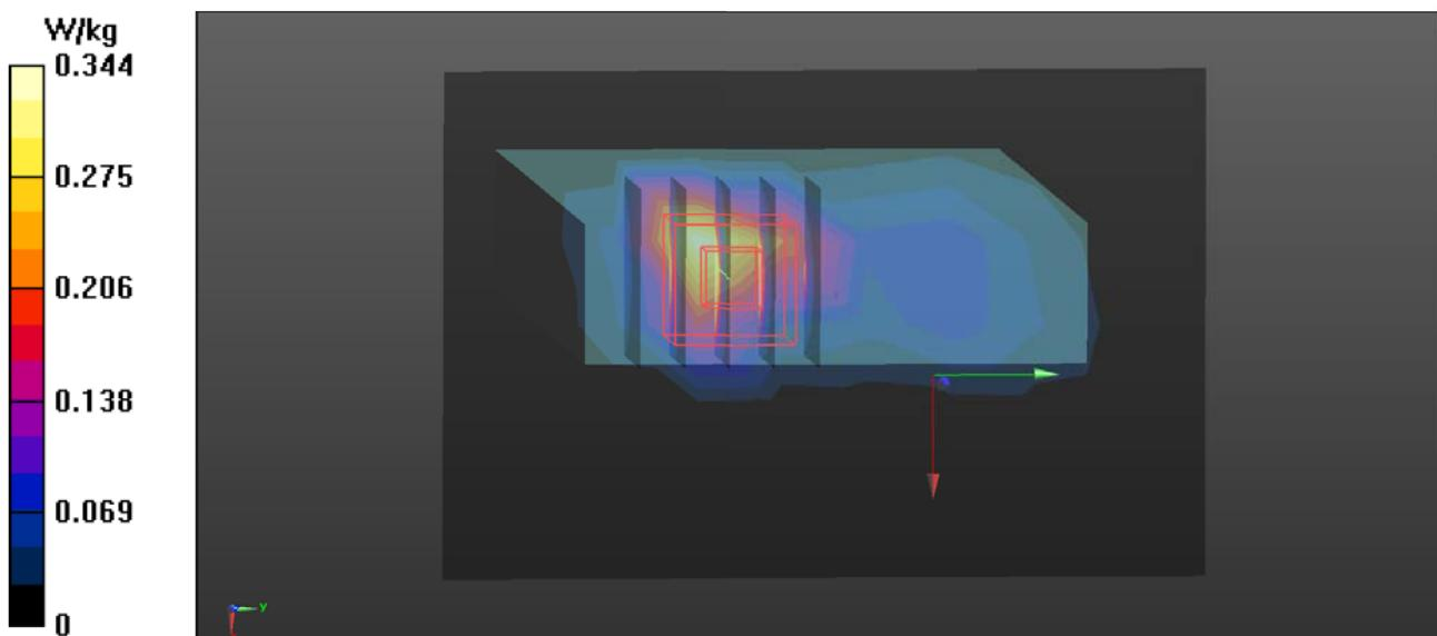
**T56 802.11n\_HT40\_Ch38\_Left Side\_0.5cm\_Ant 0+1****DUT: FIH;**
