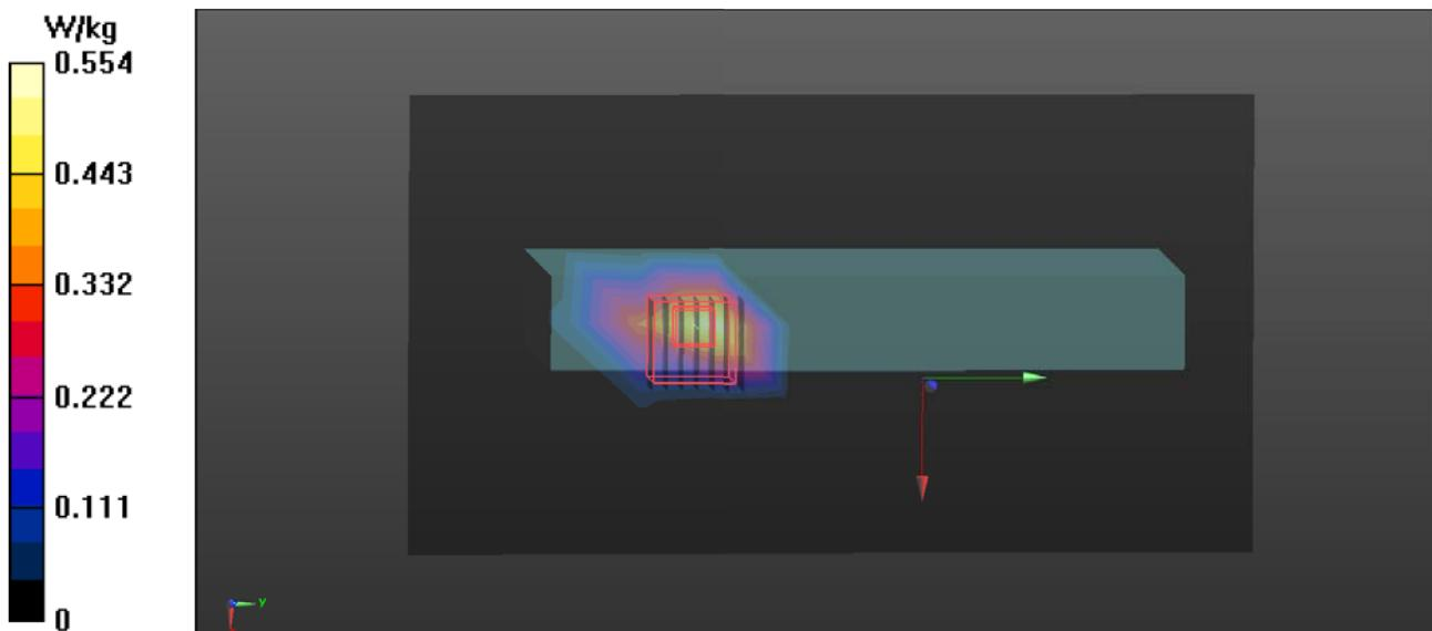
**T16 802.11n\_HT20\_Ch52\_Bottom Side\_0.5cm\_Ant 0****DUT: FIH;**
