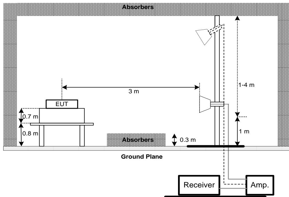
(C) For radiated emissions below 30MHz
