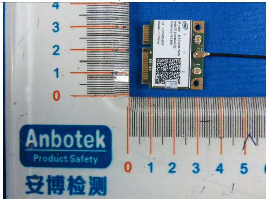
16. Figure PCB of the EUT-Front View (WiFi Module)
