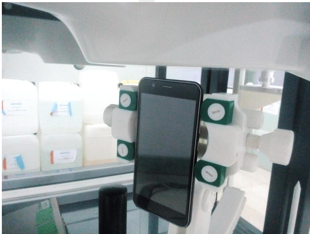
Body top side(separation distance is 10mm)
