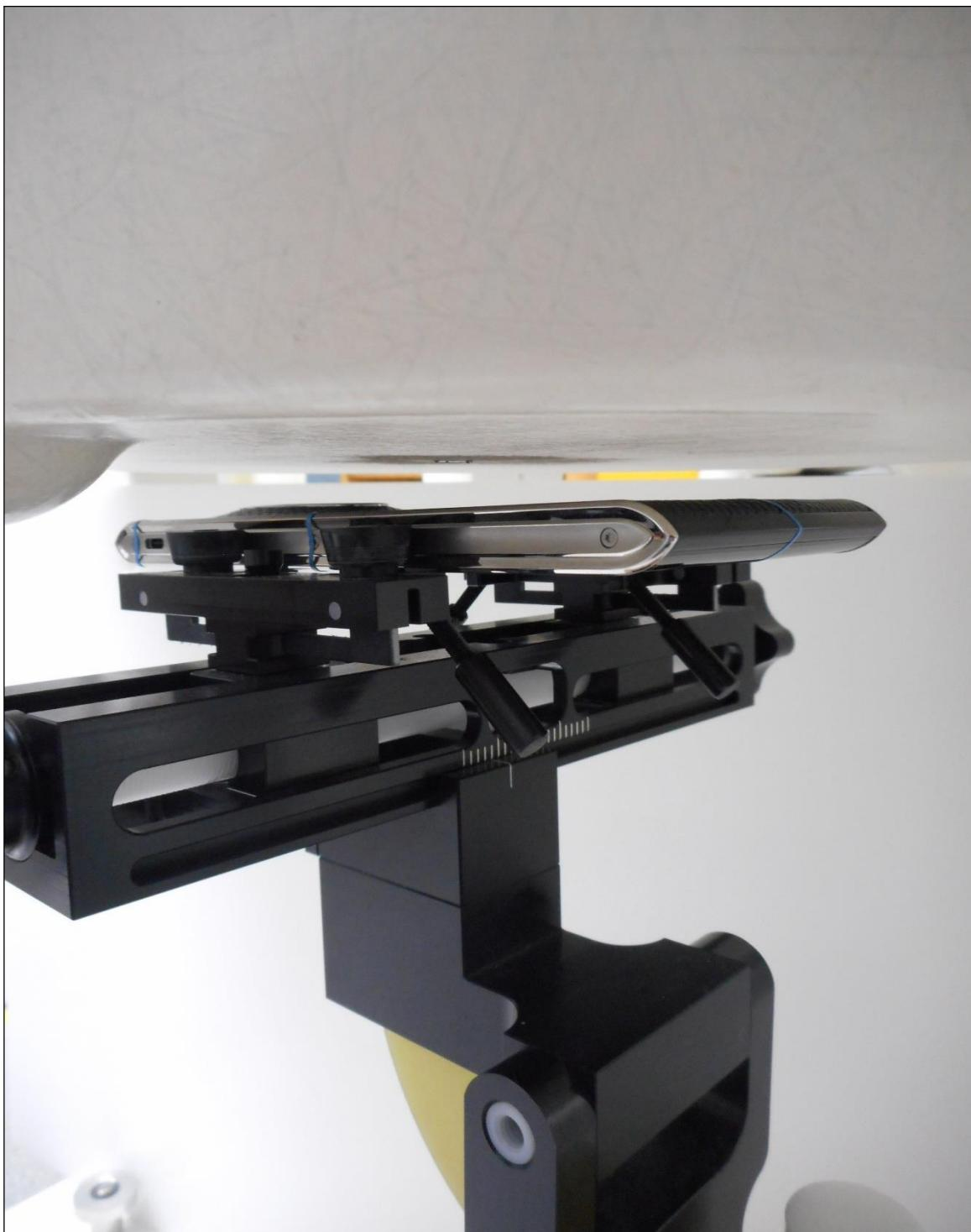
PHT/009: Back of EUT at 15mm
