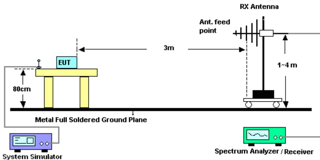
For radiated test above 1GHz
