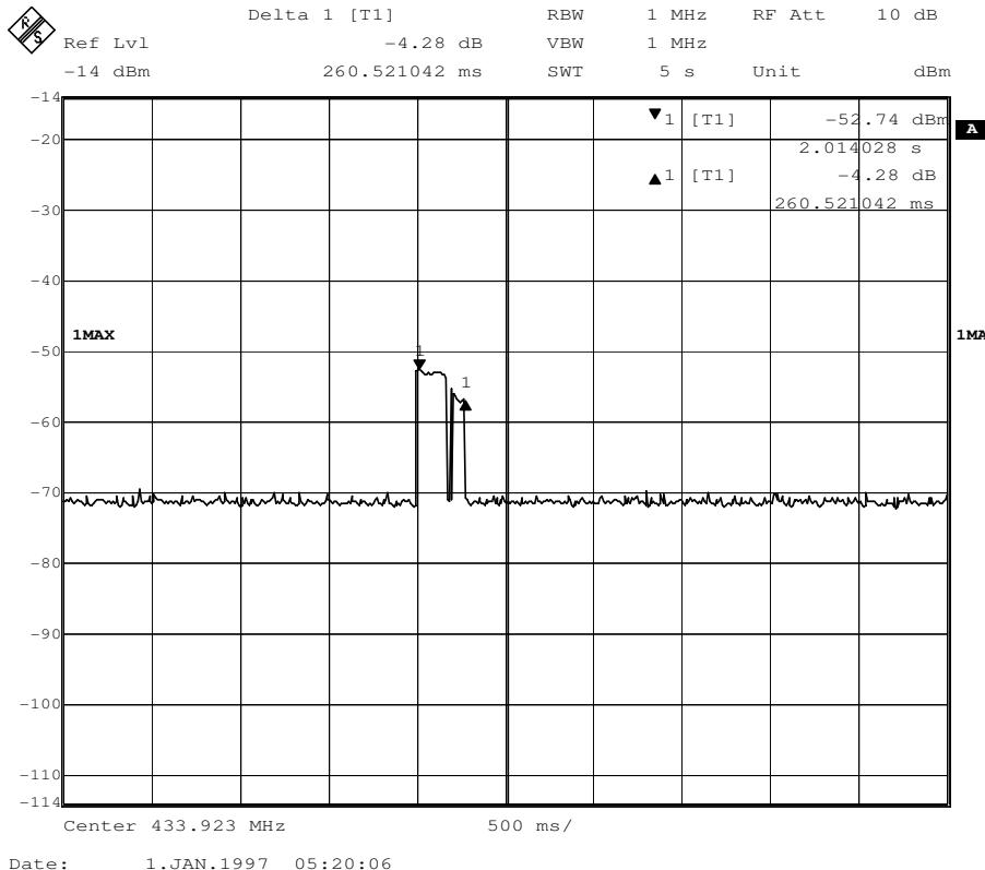
**3. Regulation 15.231 (a2)** A transmitter activated automatically shall cease transmission within 5 seconds after activation.
