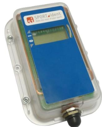
The SPORTident Station BS11-BS comes in a housing at the size of the SI-station BSx7. The station works battery powered standalone but can be controlled and also be charged by USB interface.
