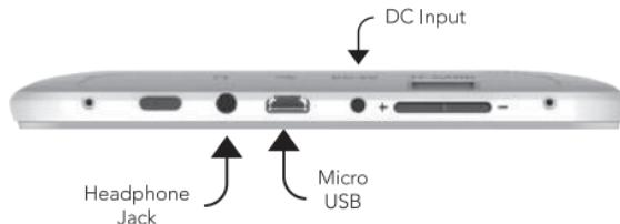
**Please note the DC Jack and the microUSB cannot be plugged in at the same time, it may damage the tablet**
