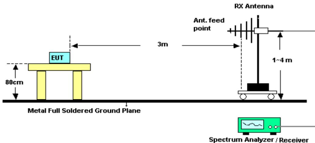
For radiated emission from above1GHz
