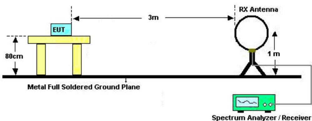
For radiated emission from 30MHz to1GHz
