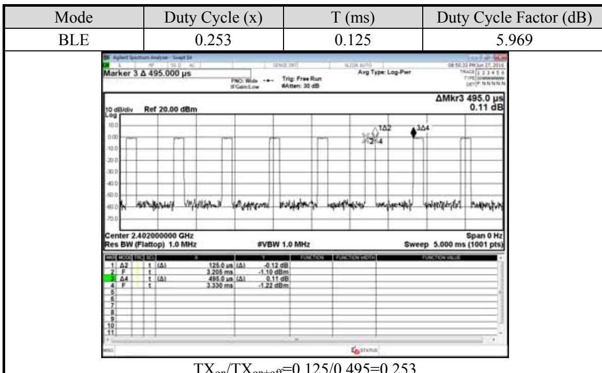
Note: When duty cycle is less than 98% (0.98) that duty cycle factor  $10\log(1/x)$  is needed to add in conducted test items measured in average detector.
