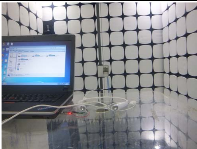
Radiated Spurious Emissions Test Above 1GHz
