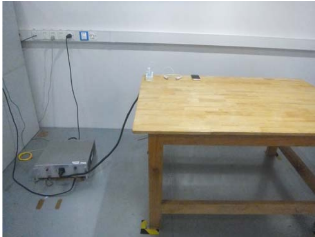
Conducted Emissions Test Setup – Front View
