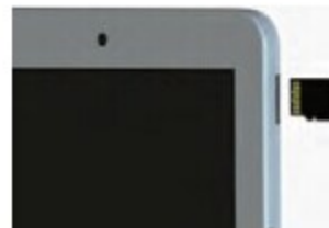
Figure 4. Inserting and Retrieving a Micro SD Card
