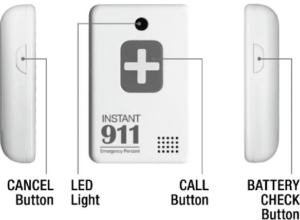
green. If the LED light is not on, recheck the position of the batteries and repeat until green light is on.
