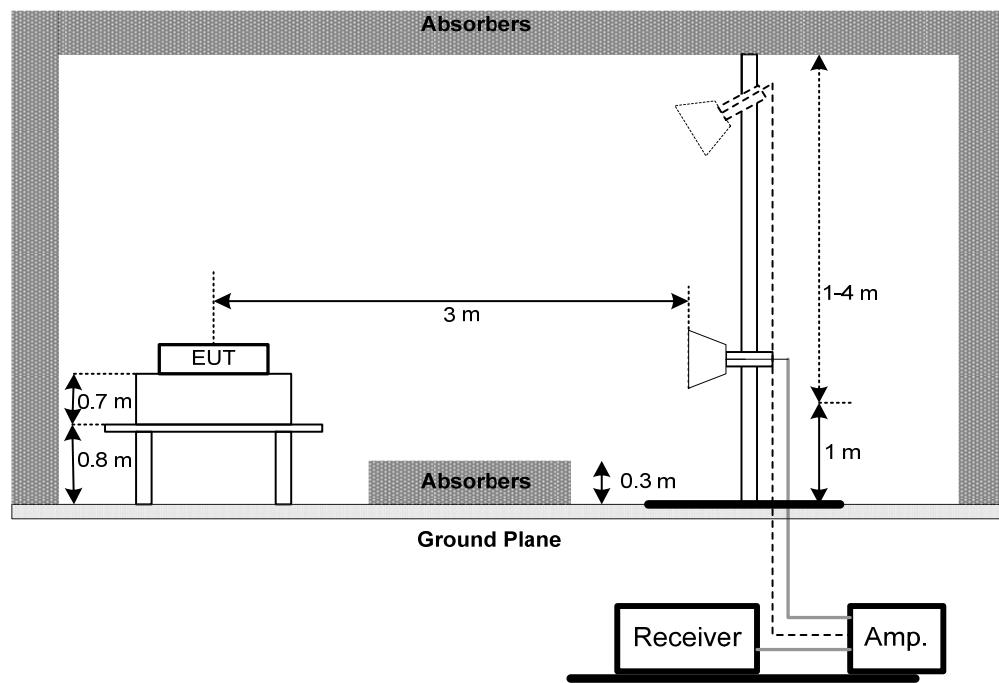
(C) For radiated emissions below 30MHz
