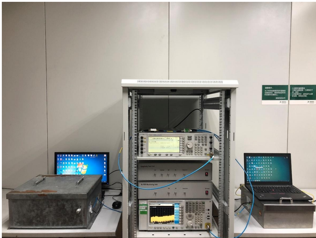
DFS Set-up Photo: Slave and Spectrum Analyzer
