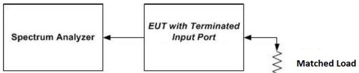
Uplink noise power measurement in the presence of a downlink signal
