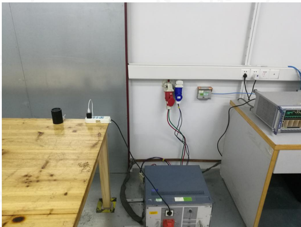
RADIATED EMISSION TEST SETUP BELOW 1GHZ
