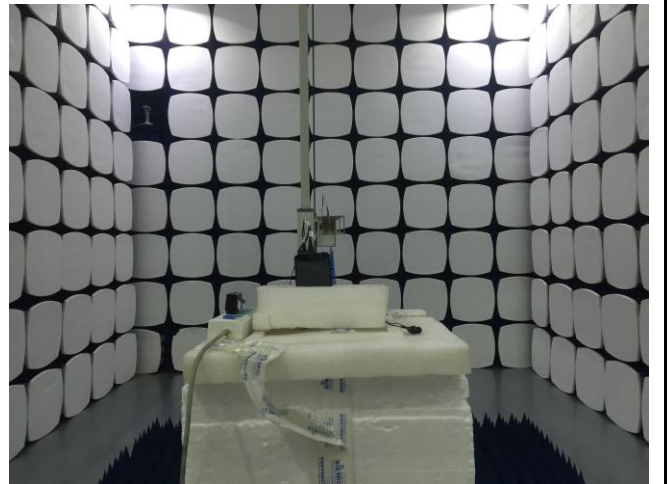
Radiated Spurious Emissions Test Setup Above 1GHz
