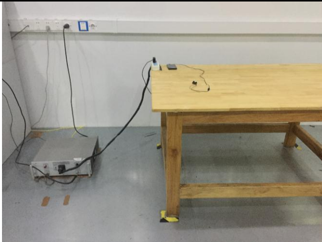
Conducted Emissions Test Setup Front View
