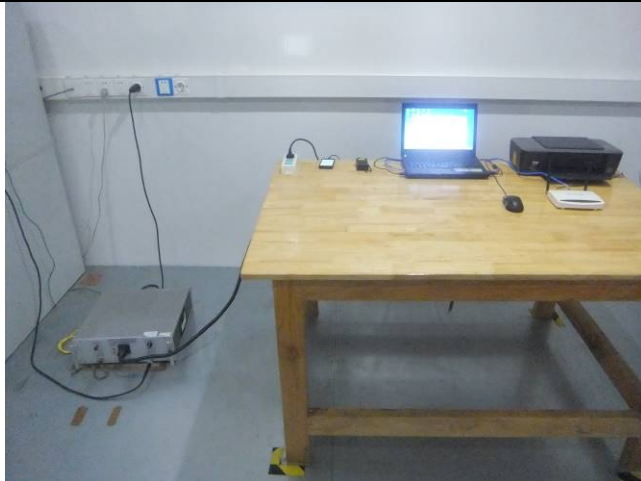
Conducted Emissions Test Setup – Front View
