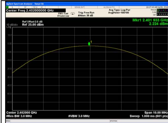
GFSK Output power - Low CH 2402
