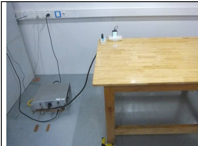
Conducted Emissions Test Setup Front View
