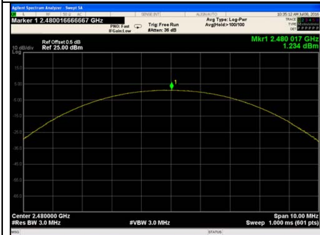
8DPSK Output power - High CH 2480
