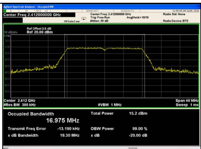
802.11g 20dB Bandwidth - Low CH 2412
