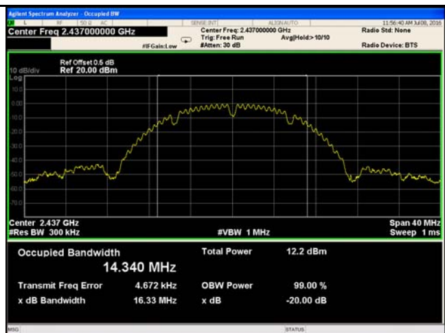
802.11b 20dB Bandwidth - Mid CH 2437
