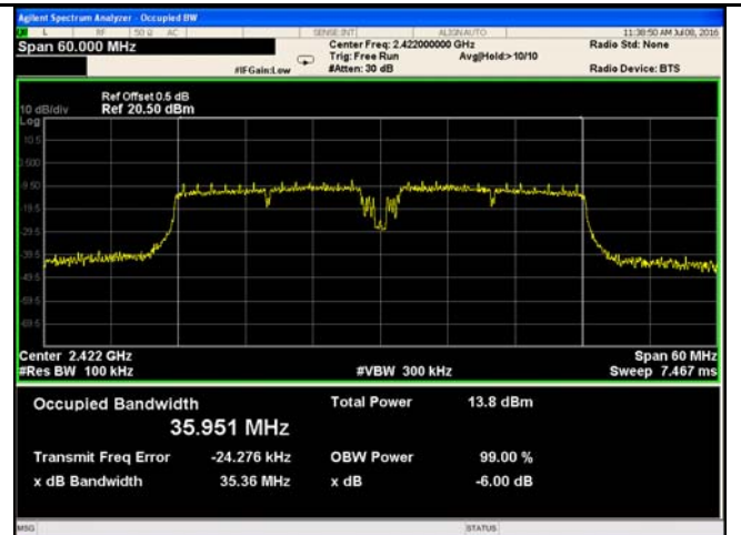
802.11n40 6dB Bandwidth - Low CH 2422
