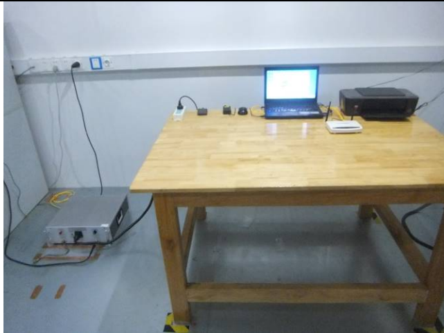
Conducted Emissions Test Setup – Front View
