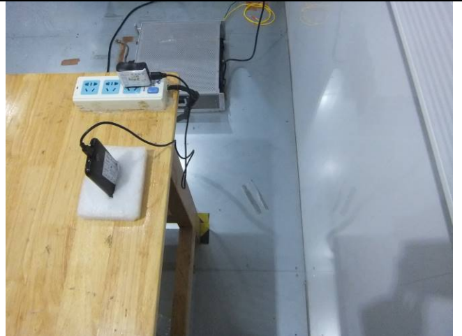
Conducted Emissions Test Setup Side View
