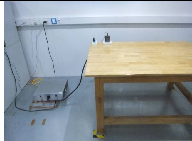
Conducted Emissions Test Setup Front View
