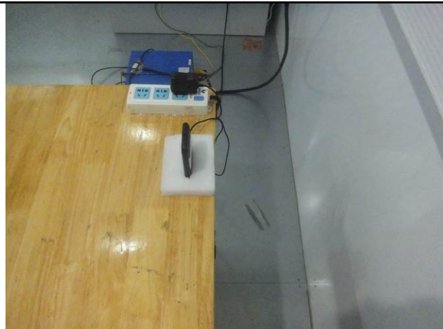
Conducted Emissions Test Setup Side View
