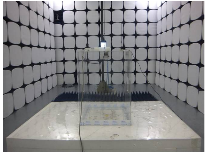
Radiated Spurious Emissions Test Setup Above 1GHz
