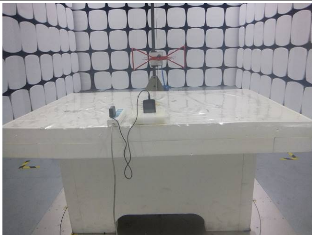
Radiated Spurious Emissions Test Setup Below 1GHz
