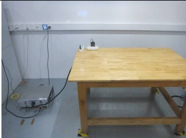
Conducted Emissions Test Setup Front View
