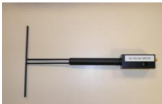
Figure 1 – Satimo COMOSAR Validation Dipole
