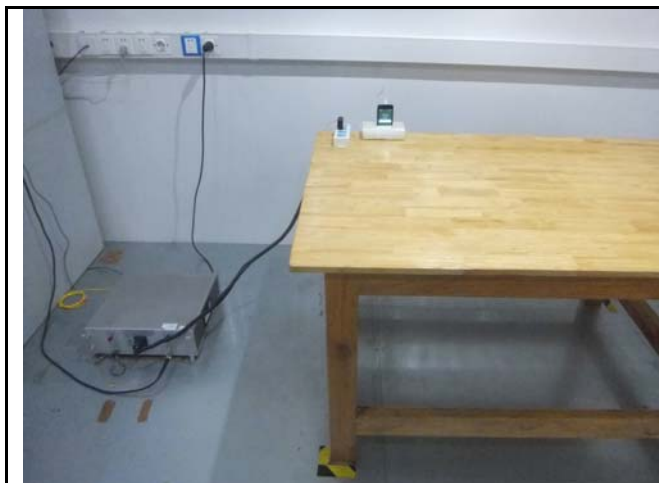
Conducted Emissions Test Setup Front View
