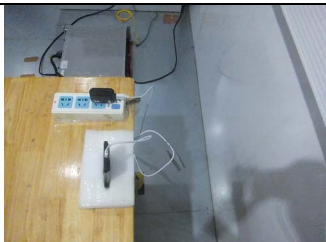
Conducted Emissions Test Setup Side View
