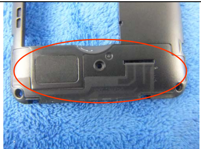
GSM/PCS/UMTS-FDD Antenna View
