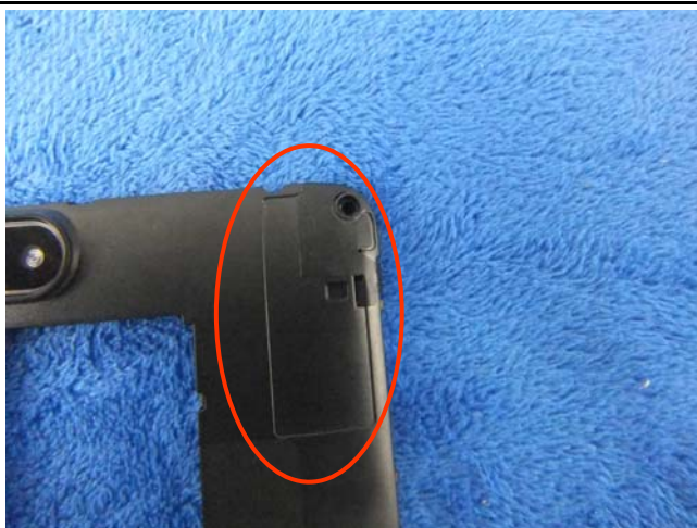
WIFI/BT/BLE/GPS - Antenna View
