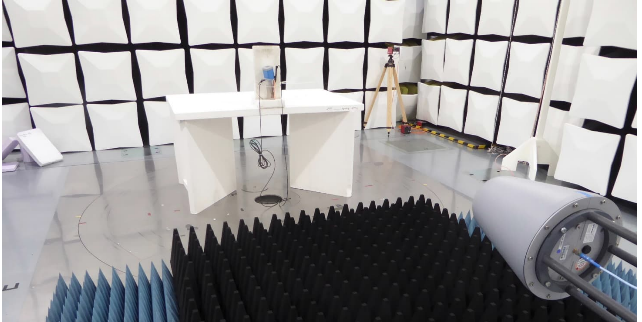
EUT nominal Position – standing Test setup semi-anechoic chamber with ground absorber M276 Preliminary and final measurement
