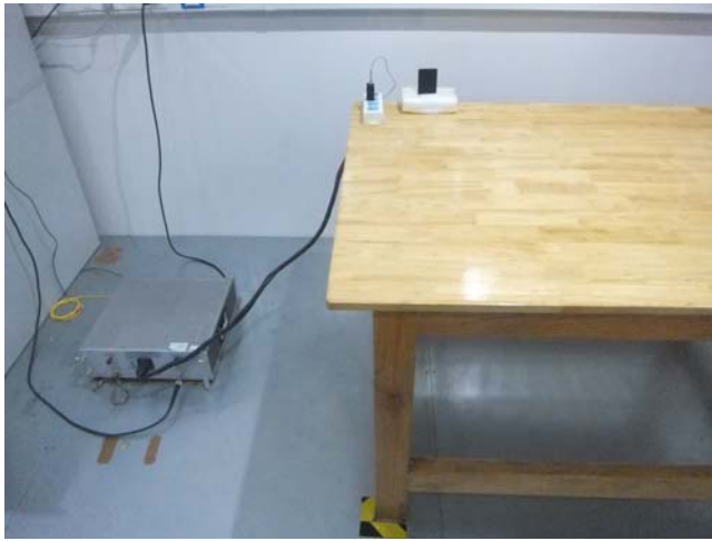
Conducted Emissions Test Setup – Front View
