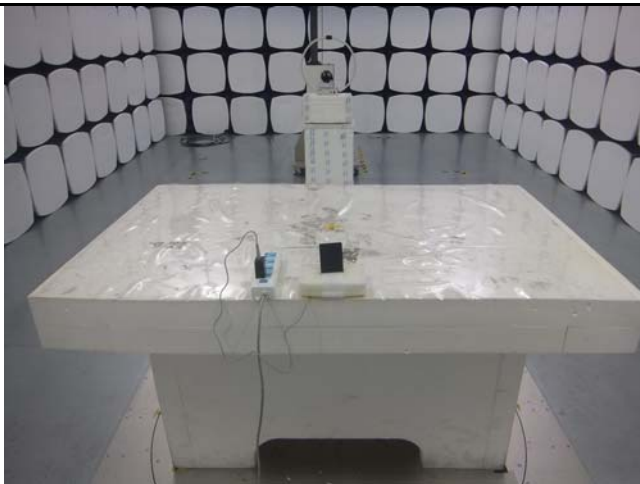
Radiated Spurious Emissions Test Setup 0.1MHz-30MHz
