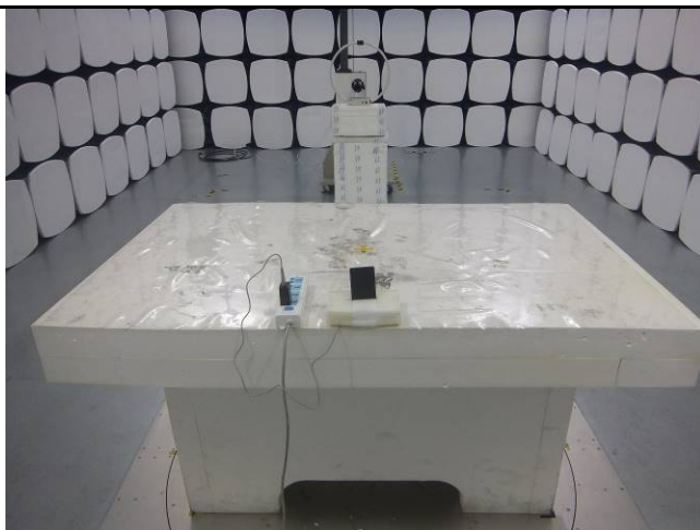
Radiated Spurious Emissions Test Setup 0.1MHz-30MHz
