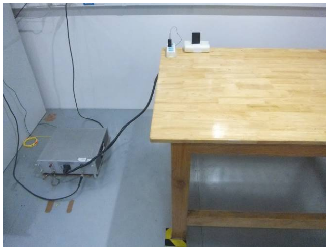
Conducted Emissions Test Setup – Front View
